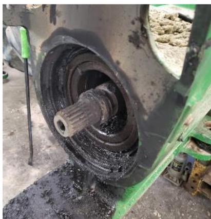
The male component of the gudgeon and the housing – no damage done!
