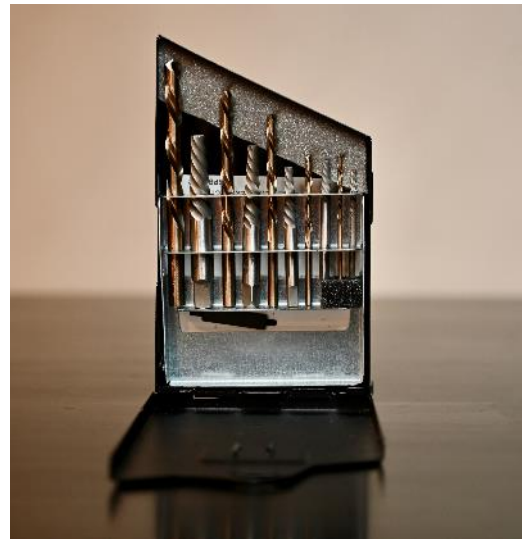
Left Handed Drill Bit and Extractor Kit
